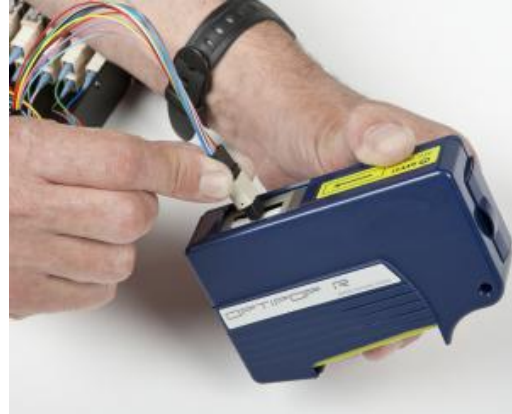
LANmark-OF MPO Cassette cleaning tool P/N: N890.125
