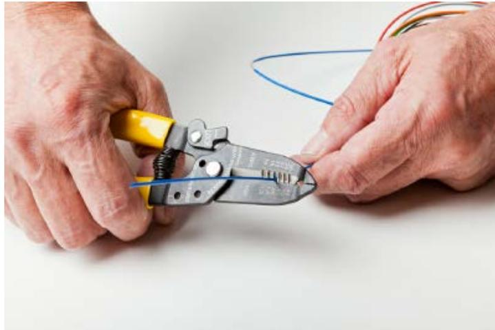
Micro-Bundles contain a small amount of jelly. The fibres shall be carefully cleaned using an appropriate degreaser before termination.
