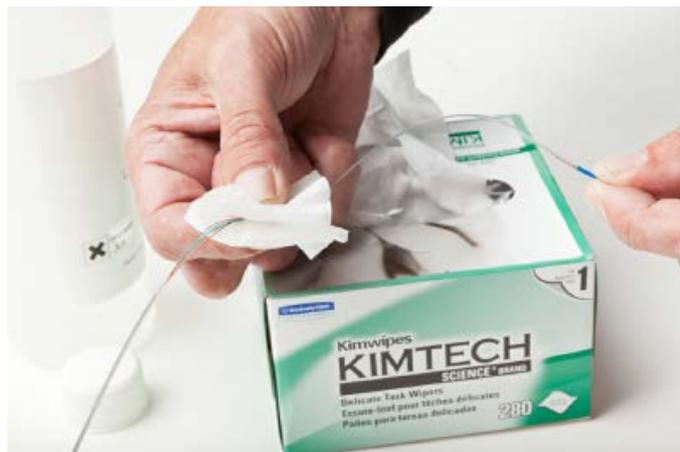
4. Split the fibres and repeat the cleaning process until each fibre is perfectly clean
