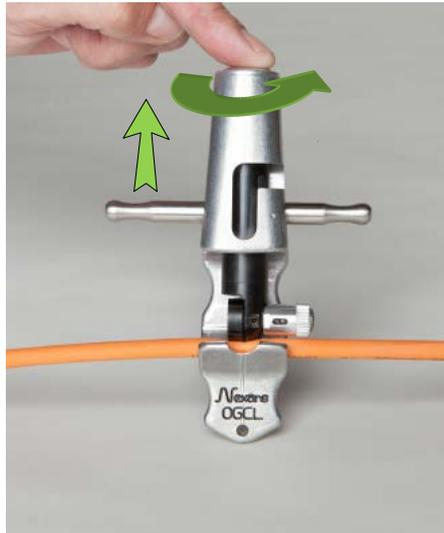
5. Install the tool on the cable with the blade located at the end of the longitudinal cut and rotate the tool around the cable to cut the jacket
