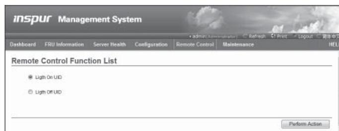
Select <Light on UID> option and click <Perform Action> to execute. After that, ID light of front and back panel of corresponding server will be on.
