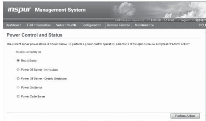
Server Power Control menu: displays the current power state of server, providing reset server, power off server immediately, power off server orderly, power on server and power cycle server. After selecting the option to execute, click <Perform Action> to execute.
