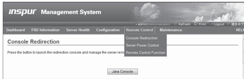
This function menu allows you to perform various remote operations on the server, including operating remote console, system switch and other control operations.
