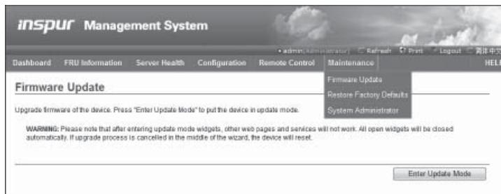
This function menu can realize remote update of BMC firmware and restart of IPMI card.
