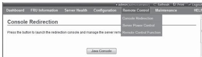
This section allows you to perform various remote operations on the server, including operating remote console, system switch and other control operations.
