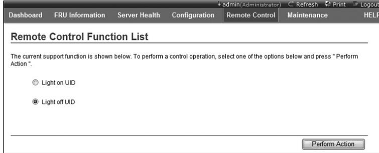
Select <Light on UID> option and click <Perform Action> to execute. After that, ID light of front and back panel of corresponding server will be on.
