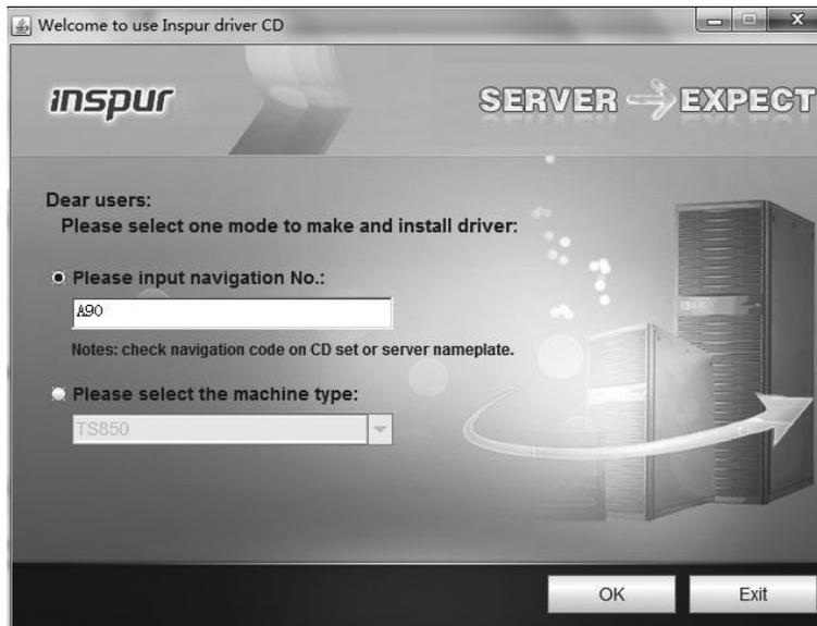
The user can select mode “Please input navigation No.” or “Please select the machine type” to make and install driver. In “Please input navigation No.” text box, input navigation No (check navigation No. on CD set or name plate), or select the specific product model in drop-down menu of “Please select the machine type”. Click <OK> to log in the interface of making driver. Click <Exit> to log out.
