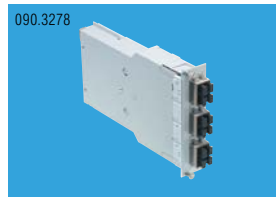
090.3278 MPO Modul 7HP, metal, MTP12-female - 6xSC-Duplex, OM4, PC/PC, ceramic, type A, серый Артикул - R514581
